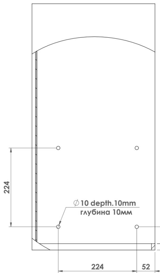
Drill sides as shown in the drawing here to the side a 9.5mm tip. The holes must have a depth of 10mm.
