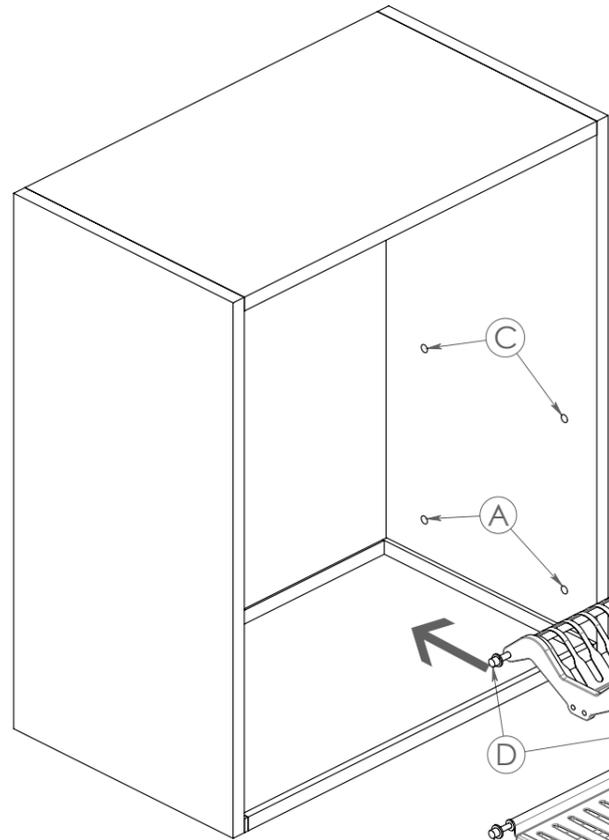
Press the pins (B) of the cup holder and hold them down insert the drawer in the cabinet.
