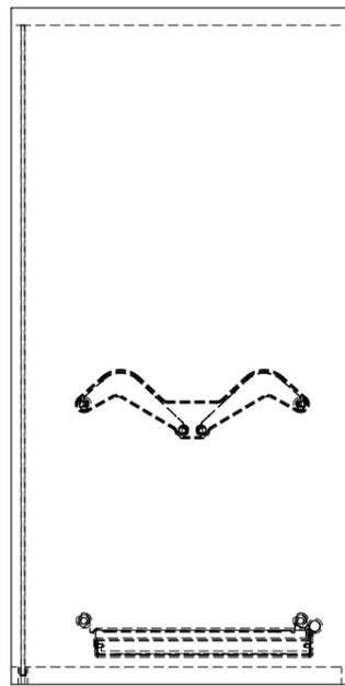
Make sure the pins are fully inserted in the holes sides of furniture.
