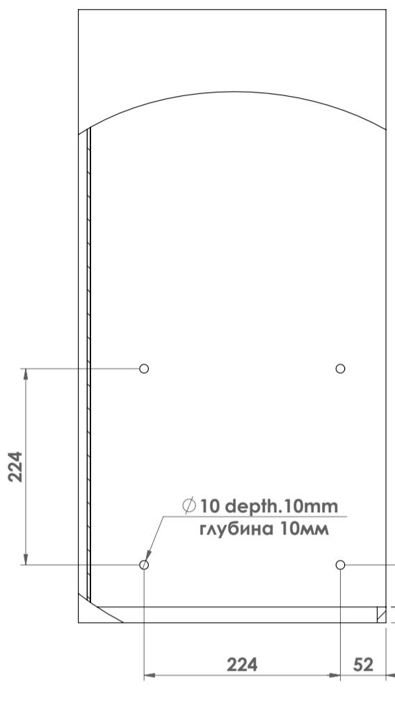
Drill sides as shown in the drawing here to the side a 9.5mm tip. The holes must have a depth of 10mm.
