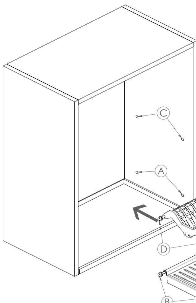
Press the pins (B) of the cup holder and hold them down insert the drawer in the cabinet.
