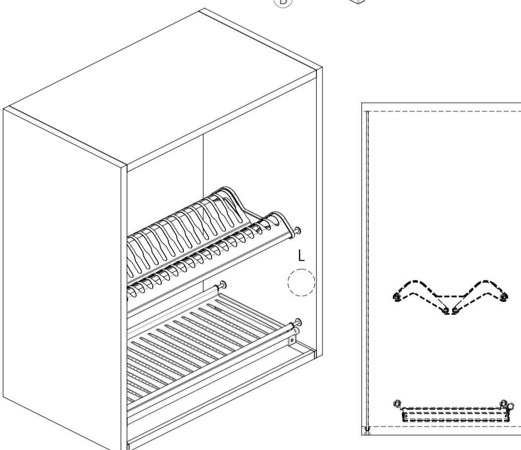
Make sure the pins are fully inserted in the holes sides of furniture.
